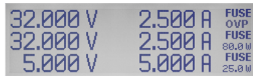
Figure 4-6: Overvoltage protection (example R&S HMP2030)
