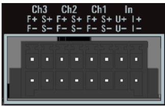
Figure 5-5: Terminal block with connector assignment
