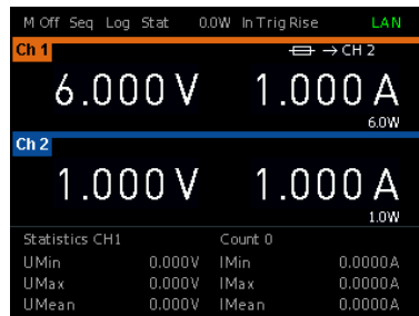
Figure 5-7: Linking of channel 2 to channel 1
