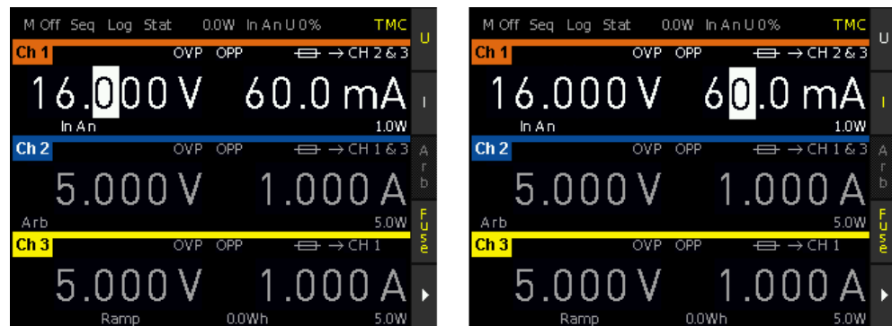
Figure 5-2: Voltage and current settings in the instrument
