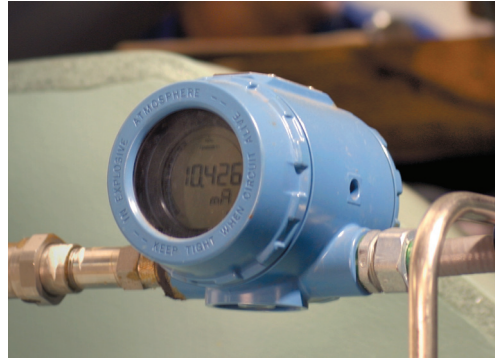
Figure 3.1.3.5b – Remote Mounted Transmitter with LCD
