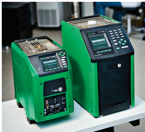
Figure 5.7.5a – Typical Field Dry Block and Metrology Grade Dry Blocks (Courtesy of Beamex)
