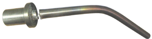
Figure 3.3.7.1a – Example of a Thermowell Failure
