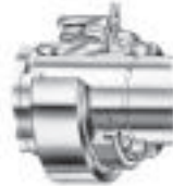
Figure 8. HMV nut and stop ring in position to press loose an adapter sleeve
