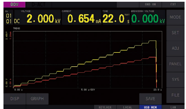
Example of stepped voltage rise testing
