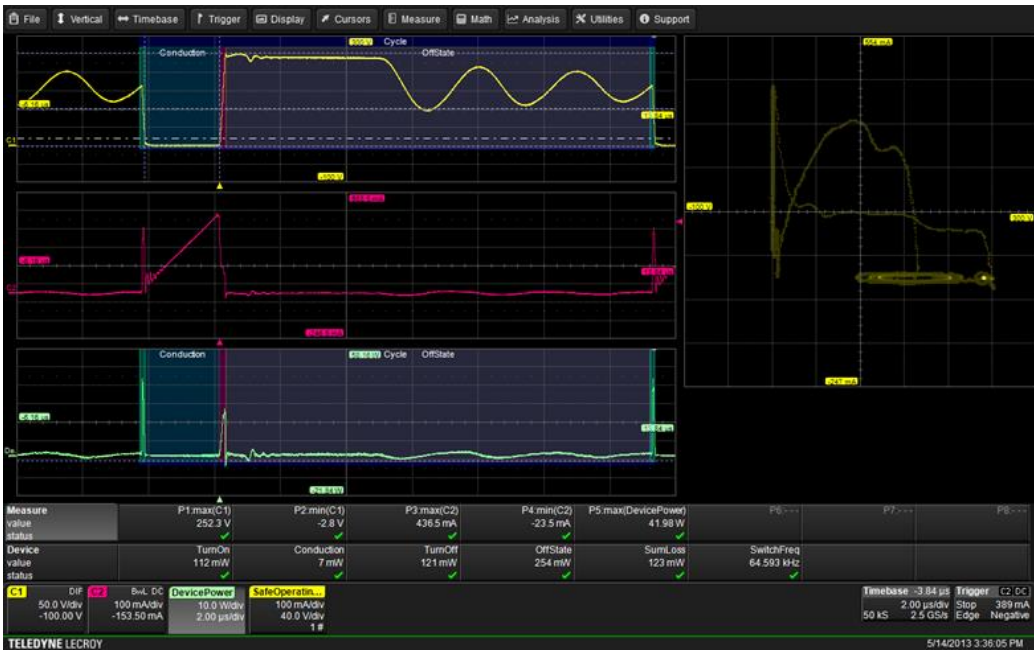
Figure 3: Using the maximum parameter to measure the maximum voltage, current, and power
