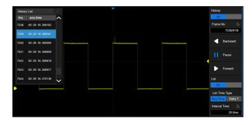
History function can record up to 80,000 frames of waveforms. The recording is executed automatically so that the customer can playback the history waveforms at any time to observe unusual events and quickly locate the area of interest using the cursors or measurements. The failed frames of the Mask Test can be stored as history
