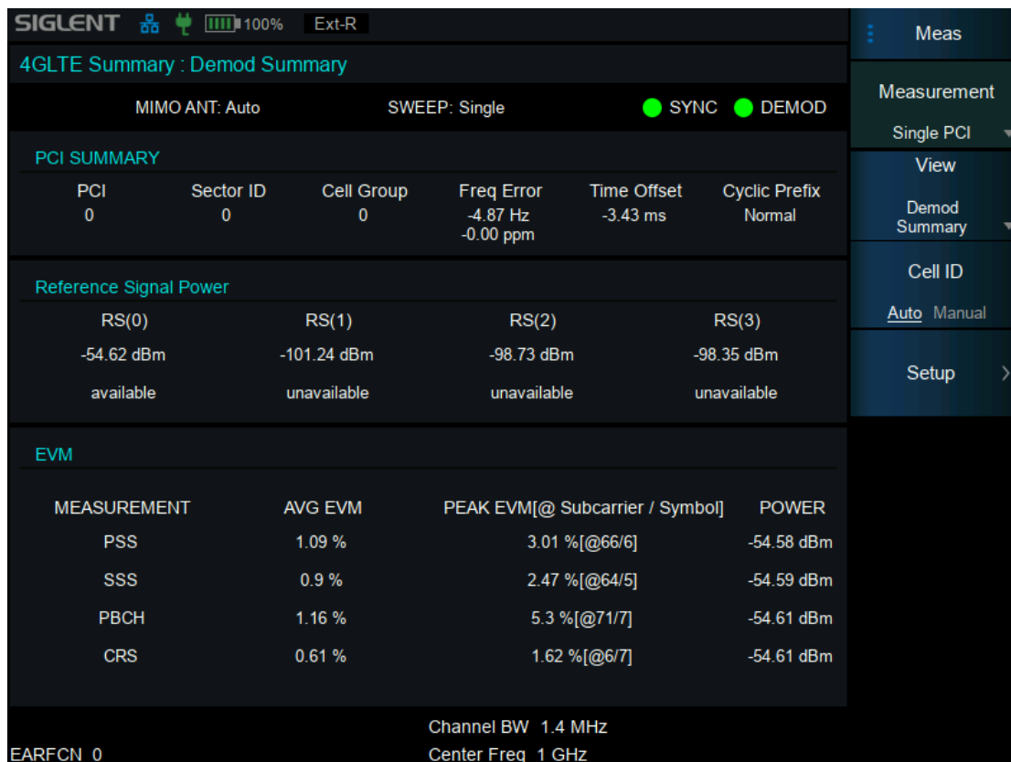
Figure 9–1 Single PCI Demodulation View
