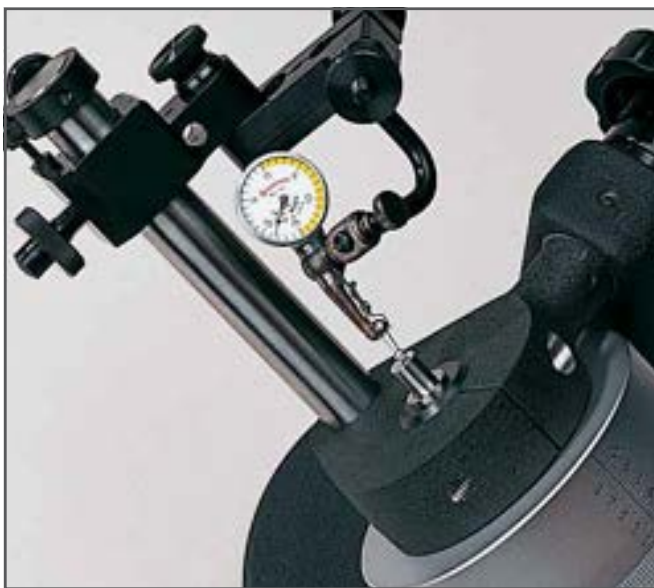
Dial test indicator held in place by an offset attachment
