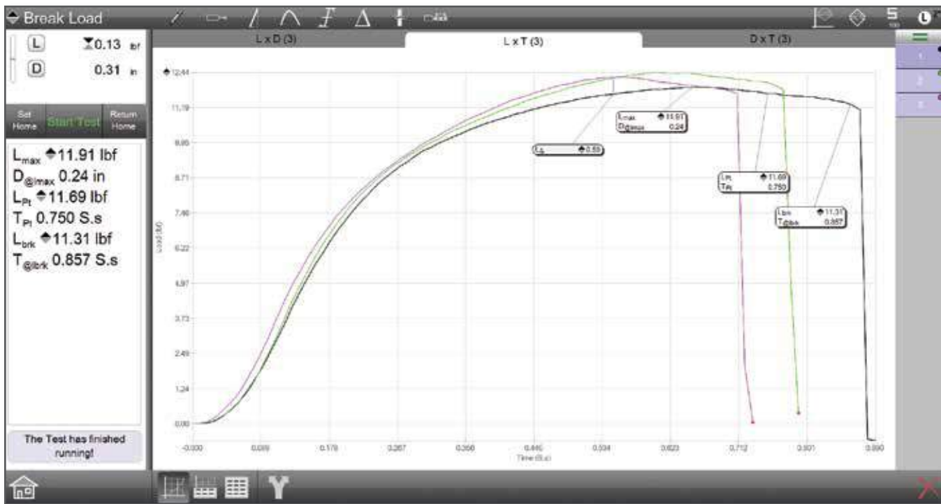
(Above) Using the "Multiview" function, you can measure using multiple graphs from your batch. Graph traces are overlaid onto one another and color-coded for identification. In this example, the delta variance is measured between the three test runs. The variance is measured at a point between the graph with the greatest value and the graph with the lowest value. This function can be used for "benchmark comparisons".
