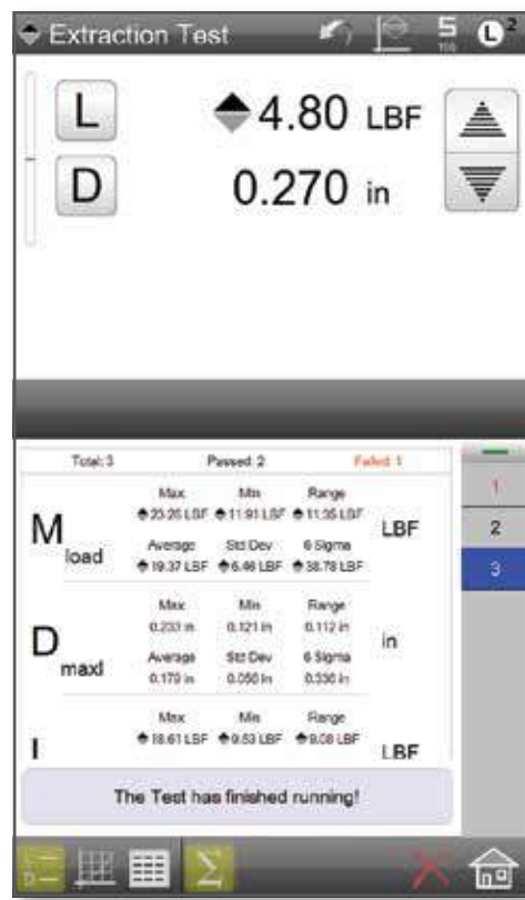
The Statistics view displays the results and their associated statistical values. The header displays the total, passed and failed test runs. Failed runs display in red.
