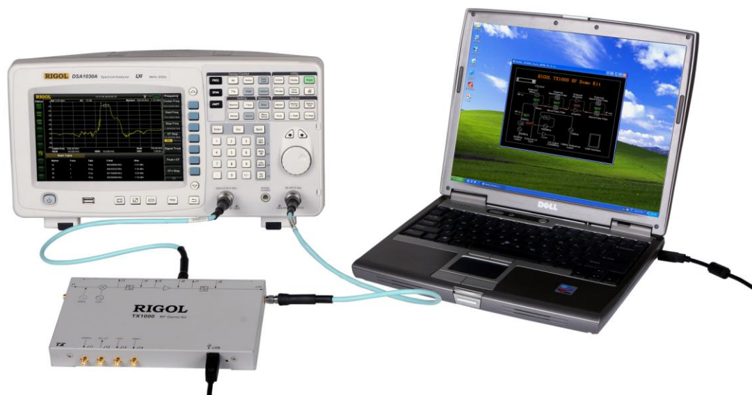
Figure 13 Testing the Characteristics of the Band-pass Filter
