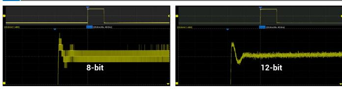
12-bit resolution shows you more details and less noise on the waveform.
