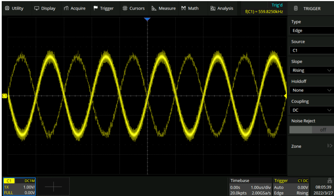
Noise Reject = Off
