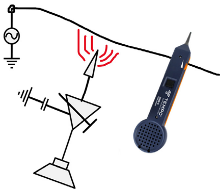
Figure 2: Using electrostatic detection in wire identification
