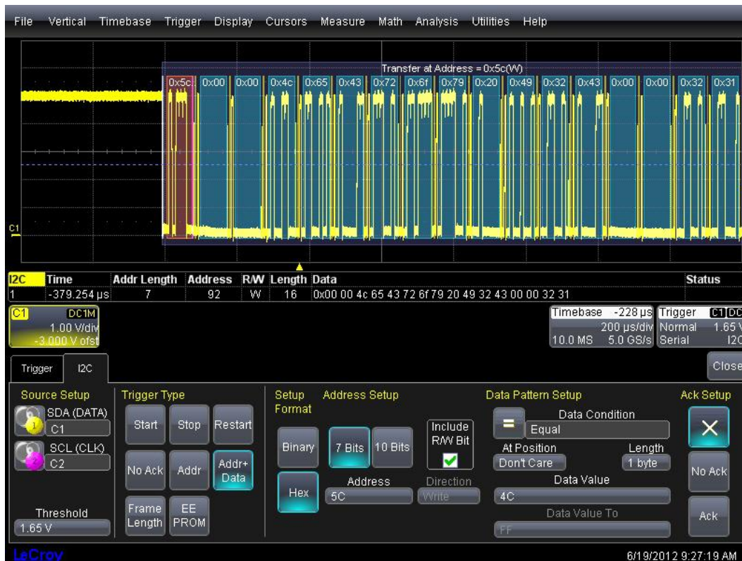
Figure 2: An I 2 C signal is captured and decoded. The trigger setup is very easy to use.
