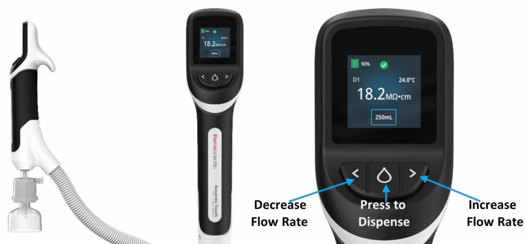
Figure 66. Aquanex Touch Smart Dispenser POU UI and Dispense Buttons
