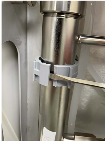
Figure 83. Using Flat-Head Screwdriver to separate the halves of the Clamps
