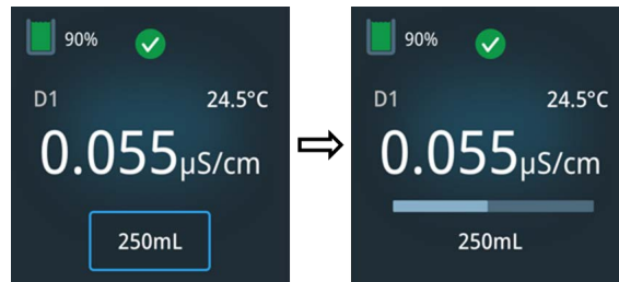
Figure 68. Aqanex Touch Screen Before and During Volumetric Dispense
