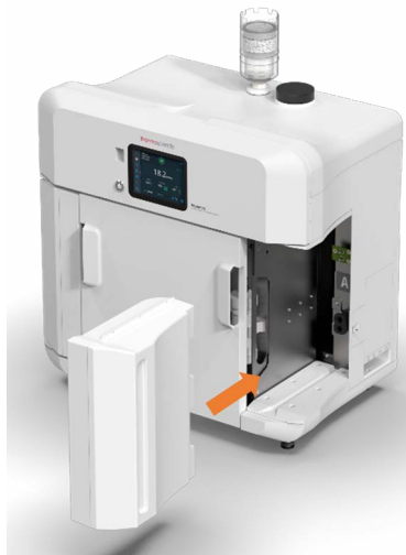
Figure 35. DI Pack Insertion in 10L Aquanex Main Unit
