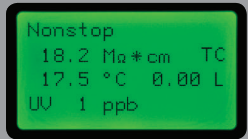
Intuitive display shows important system parameters
