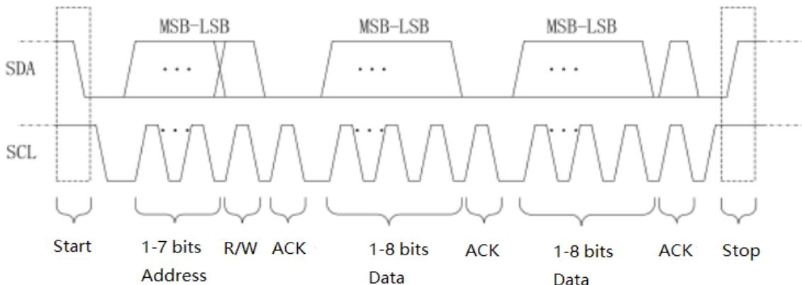
I<sup>2</sup>C trigger can set SCL source, SDA source, operating direction, trigger condition, address setting and data setting.
