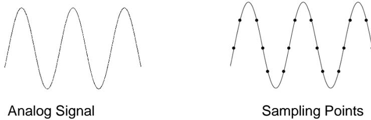
Sampling rate refers to the time interval between two sampling points. The maximum sampling rate of the UPO1000CS series is 1 GS/s.
