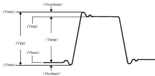
Max: The voltage from the highest point of the waveform to GND.
