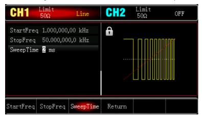
To view the shape of the linear sweep wave through an oscilloscope as shown in the following figure.
