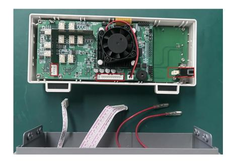
4. Remove the fan, and use a T10 Torque screwdriver to remove the four screws and the power supply cable of the fan. As shown below:
