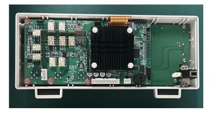
6. Carefully lift up and remove the motherboard.
