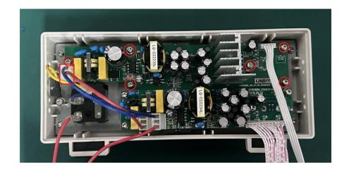
2. Remove the power module; use a T10 Torque screwdriver to remove the 5 screws and the blue wire, as shown in the figure below:
