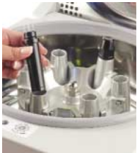
C8600-34 Microhematocrit tube adapters hold up to four tubes each. Supplied in a Pk/2.
