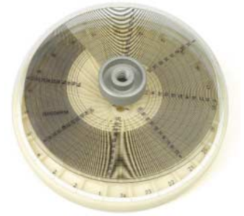
24 place rotor for capillary Microhematocrit tubes. Hematocrit Reader incorporated into the cover
