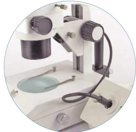
Light source shown installed at rear of base in correct position for IVF. This position is transmitted (bottom) illumination.
