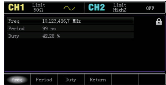
High-precision frequency meter, which can measure the frequency range of 100mHz–200MHz.
