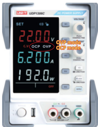
Over voltage/current/temperature protection
