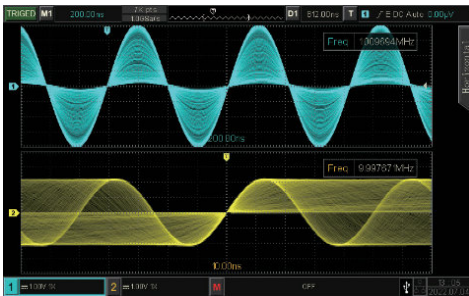
Multi-Scopes technology, which can be used for testing signals with different clock sources and different frequencies
