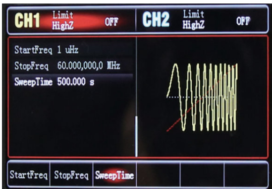
Sweep function; Scan type: linear and logarithmic, test scan from low to high, and scan output from high to low
