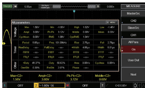
Automatic Measurement of Waveform Parameters
