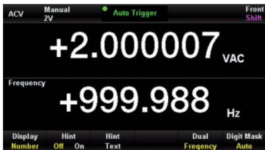
Display main and auxiliary parameters on the same screen.
