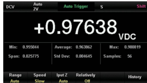
Various mathematical operations: maximum, minimum, average value, standard deviation, pass/fail, dBm, dB, relative measurement, histogram, trend chart, bar chart
