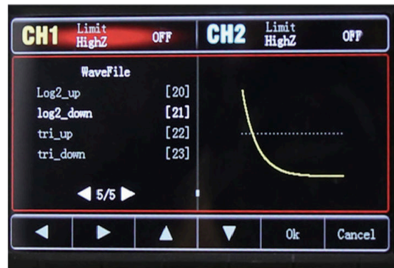
Built-in 24 arbitrary waveforms. 4kpts digital arbitrary waveform storage
