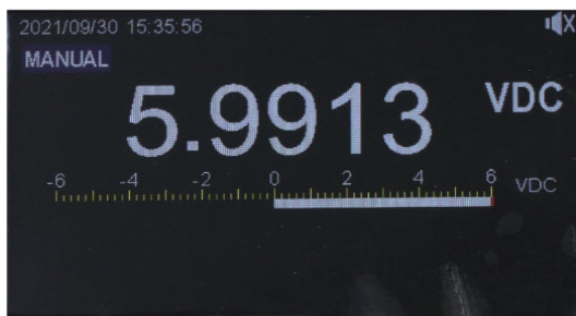
Analog simulation bar makes the display of measurement results more intuitive.
