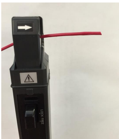
Figure 4: A test for dV/dt sensitivity
