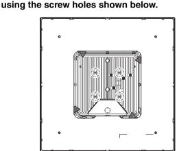
3. Attach the VESA mounting bracket to the ceiling.
