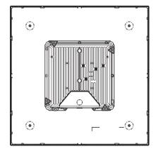
3. Install the unit by attaching it to the wires hanging from the ceiling, making sure that the unit is
