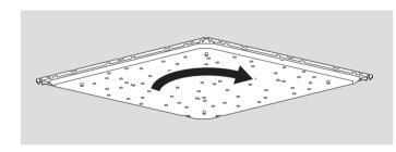
3. While holding the unit up, turn the four mounting screws clockwise with a Phillips screwdriver to tighten them.
