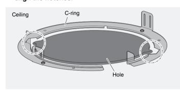
4. Secure the C-ring to the ceiling by using the mounting screws for the C-ring.
