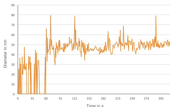
Diagram 4: Soldering with extraction – particle size.
