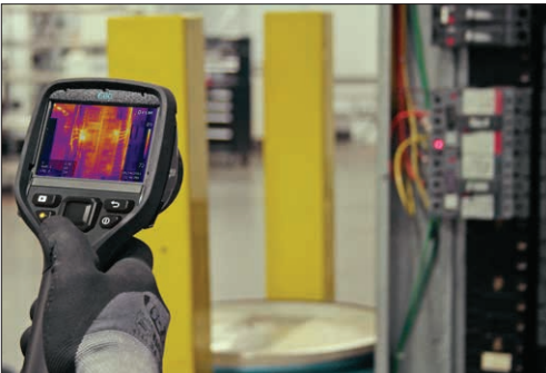
Laser pointer marks the target for visible light reference images.
