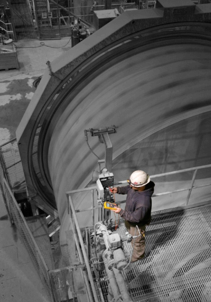
Ken Bartlett troubleshooting a flow control valve for the water addition to the Sag Mill.
