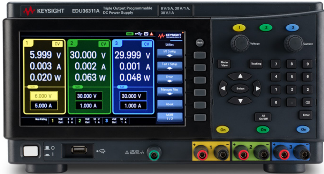
Figure 3. EDU36311A triple-output bench power supply
