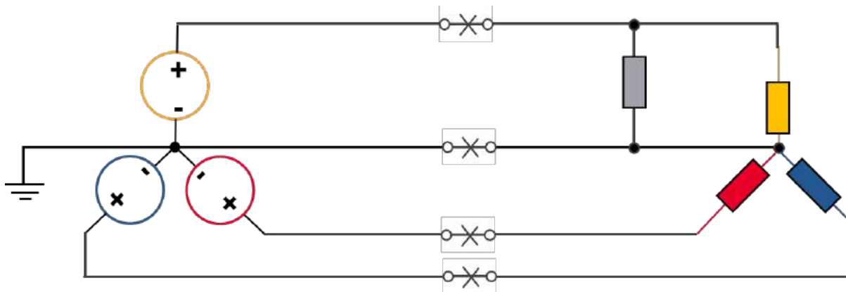
Figure 6.08. Potential failure points when driving Wye and single phase loads.
