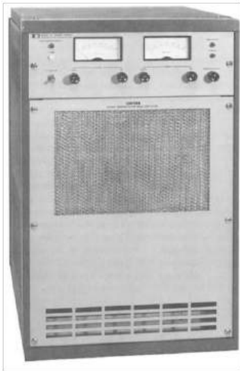
HP SCR-10 Series 10 kW power supply circa 1980 Height = ~16 U (27.75 inches; 705 mm) Weight = >500 lbs. (227 kg)
