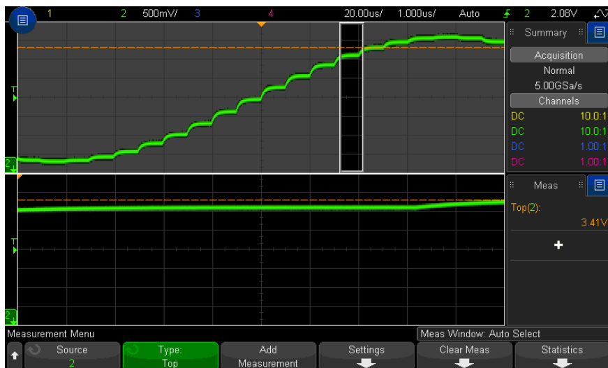
Figure 48 Isolating area for Top measurement
