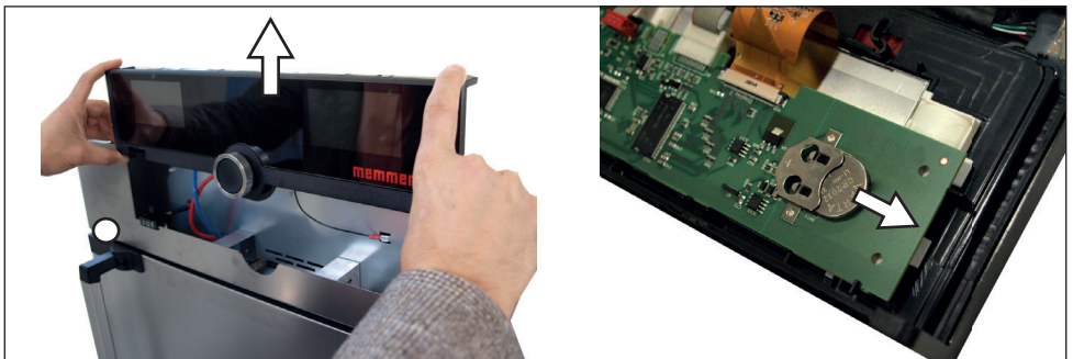
Fig. 30 Removing the lithium battery
