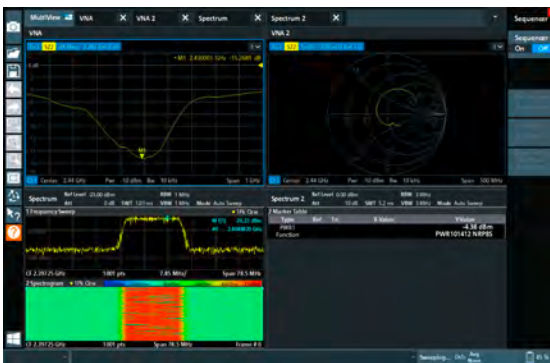
MultiView provides a convenient overview of all active R&S®ZNL modes. The figure shows a combination of spectrum analyzer and network analyzer. In this view, all modes can be updated sequentially.
