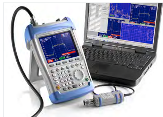
Remote control via LAN or USB: The R&S®FSH can be remotely controlled via the USB or LAN interface and integrated into user-specific programs
