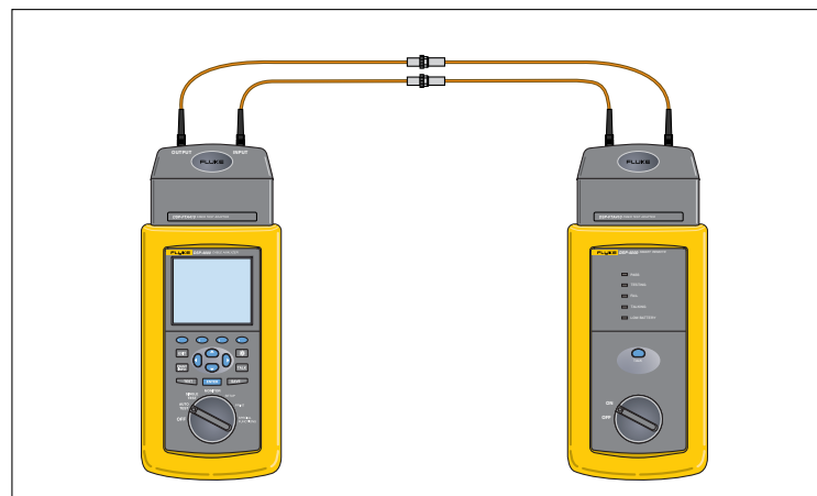
Figure 1. Reference configuration with a dual fiber tester simultaneously testing two fiber links
