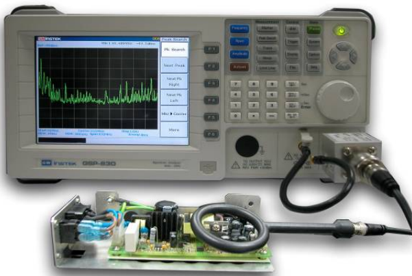
Fig. 10. Optimal solution of EMI emission Measurement
