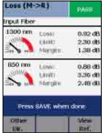
Figure 3 – Loss test results for the fiber connected to the input port on the main tester unit. The result includes the loss for both multimode wavelengths (installation test standard)
