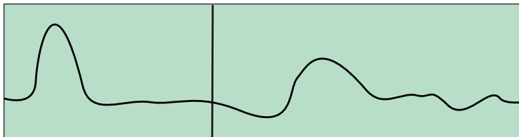
Figure 6: Water in the Cable (example)
