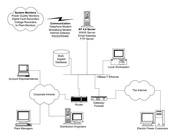
Figure 1: Advanced Configuration for a Power Quality Monitoring System
