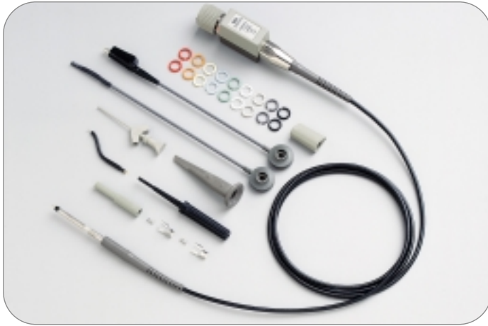
► Figure 41. A typical passive probe with accessories.
