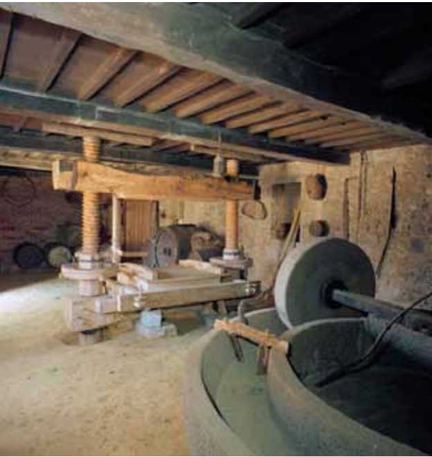
Syvret: press-house restored as a working exhibit with a new twin-screw wooden cider press (1993) and apple crusher of Chausey granite (dated 1718). View south-west. Société Jersiaise
