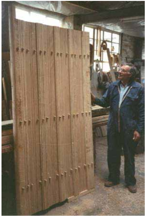
Carpenter Brian Biddle with the finished door, ready for transporting for Hamptonne. Harry Tumblety
