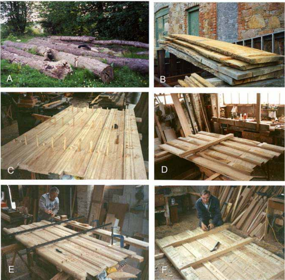
New oak carpentry: constructing a traditional harr-hung door for Hamptonne, 1991. A. Fallen oaks dragged from the woods in Rozel Valley, ready for transporting to a sawmill. B. After being planked, the boards were allowed to season naturally. C. Planks and muntins cut, moulded and fitted with trenails, ready for attaching the ledges. D. Trenching the muntins and fitting the ledges to the back of the door. E. Pegging the construction with the trenails. F. Trimming the ends of the trenails and finishing the back of the door. Harry Tumblety
