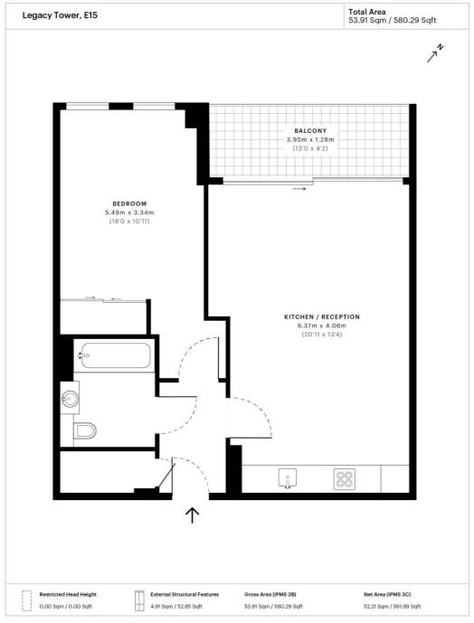
Spec floor plan captured for JLL, Stratford on 08/11/2018 using 19,534,936 laser scan points, accurate to +/- 3cm. Produced in accordance with Royal Institution of chartered Surveyors Property Measurement Standards, incorporating International Property Measurement Standard (RMS). If you intend to rely on any measurement in a transaction you should perform your own checks. Plot/Gardens illustrative only and excluded from all area calculations. SpeciD: 5be2d185d45a61118b98073e
