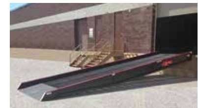
Sample warehouse yard ramp
