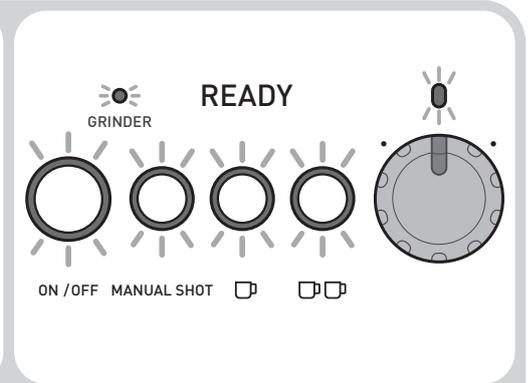
ON/OFF, EXTRACTION BUTTONS & DIAL LIGHTS all fully illuminated = Espresso Machine ready to use.
