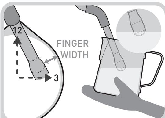
Insert Steam Wand Arm at 12 o'clock. Tip at 3 o'clock, finger width from edge and just below the surface of the milk.
