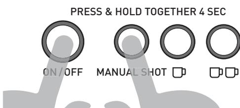
**Note:** The Cleaning Cycle can be exited at any point by pressing the ON/OFF BUTTON.
