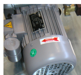
Fig. 3 Adhesive labels indicating the rotation direction
