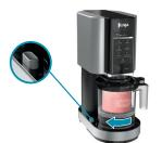
9 When the program is complete, remove the outer bowl by holding the bowl release button on the left side of the motor base and twisting the handle back to the center. As the handle is twisted, the platform will lower the bowl. Lift bowl to remove.
