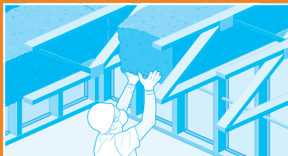
STEP 2: Insert insulation into interstitial space
