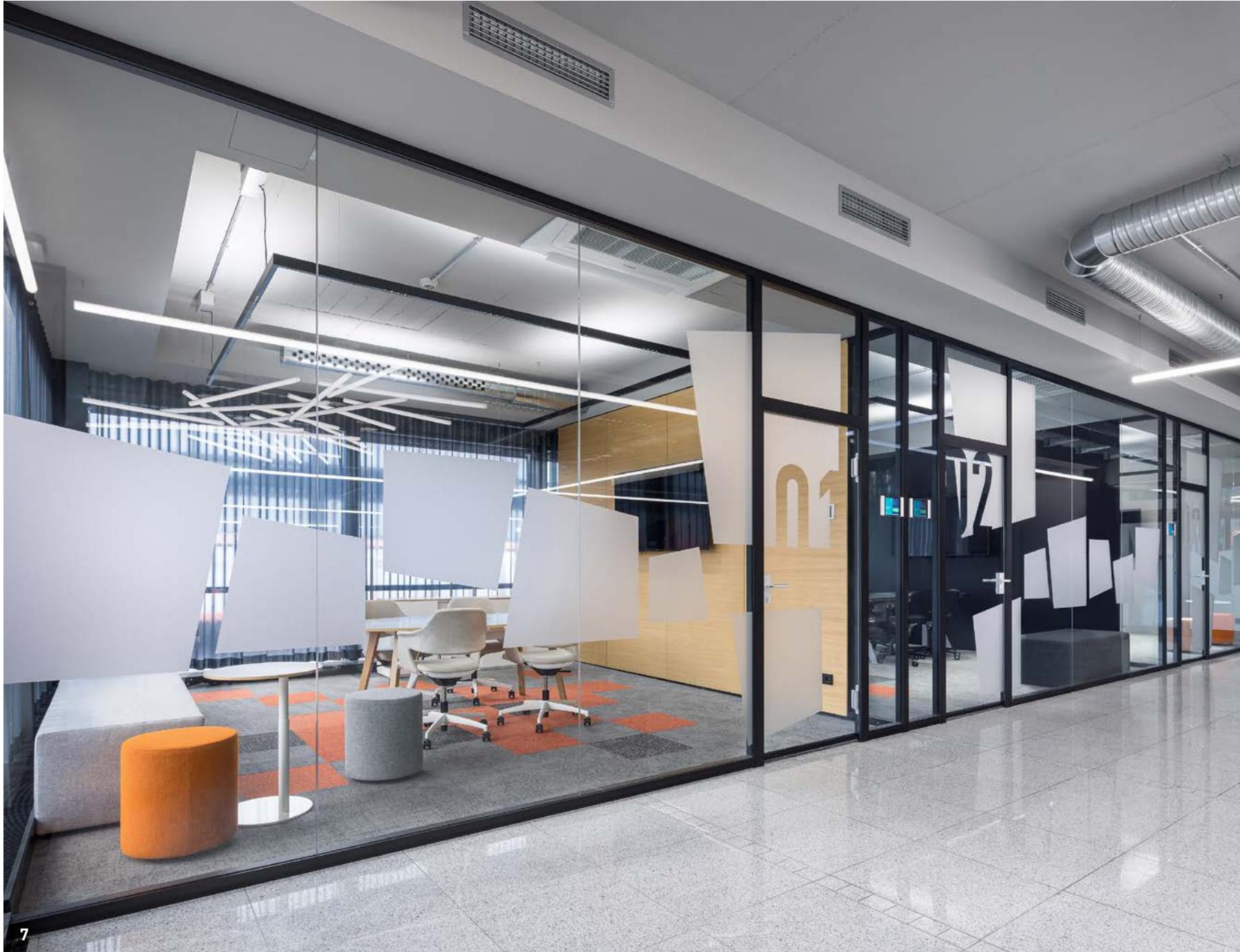
7 | Continuous look Flush glass surface with transparent glass joint.
