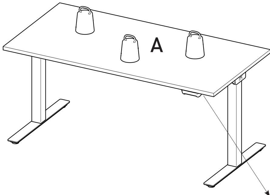
Press the release handle and move the table top to the desired position.
