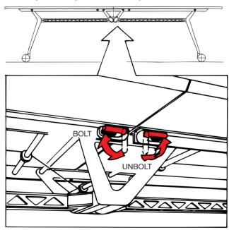
4 FINE ADJUSTMENT OF TABLE TOP POSITION possible with threaded screws.
