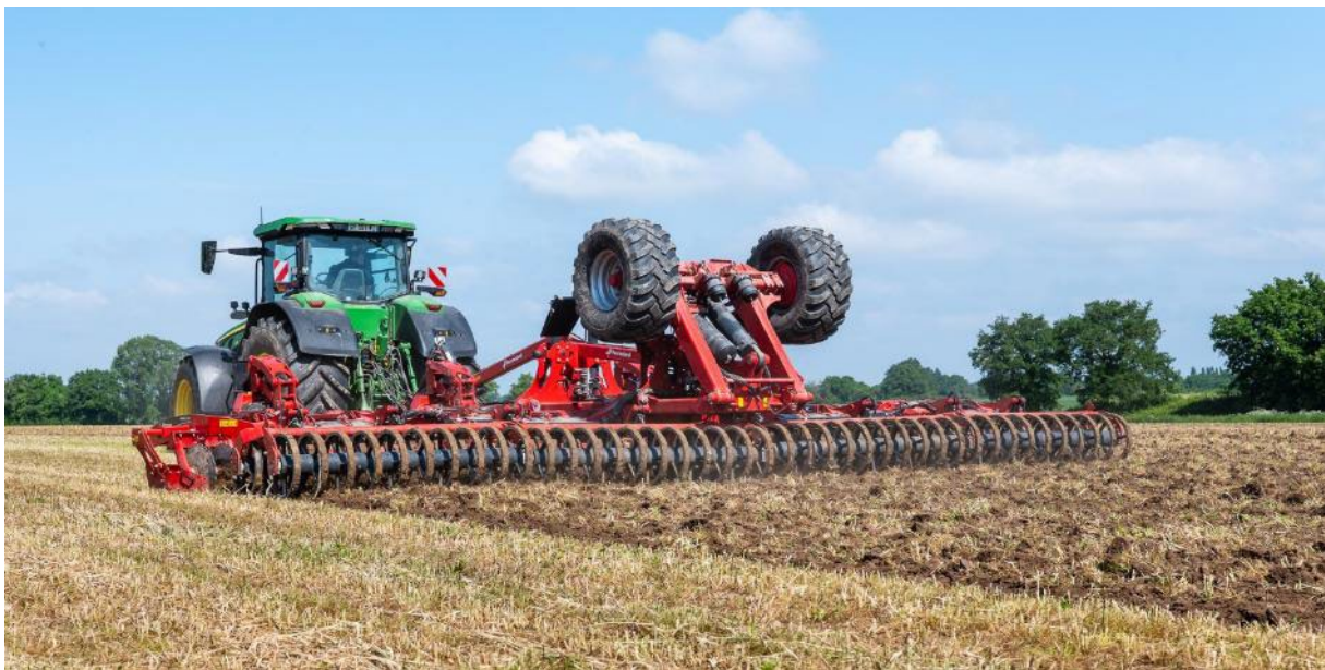
New model Kverneland Qualidisc 21103 T, large performance in working width of 10.25 meters.
