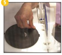
Position the replacement membrane into the retaining slot, carefully pressing the membrane into place along it's entire edge. Take special care to ensure that the location tab engages with the small pocket at the lower edge of the carrier.
