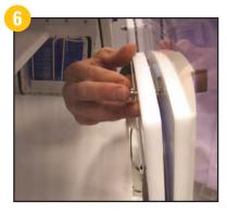
Raise the membrane carrier back into position. Tighten the screw until the carrier is firmly in place.
