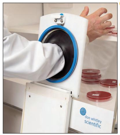
The Whitley Instant Access Porthole System is designed to provide rapid and convenient operator ingress. The flexible membrane component is very durable, but will need replacement from time to time.
